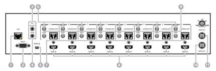
**LAN:** This port is the link for Telnet and Web GUI controls, connect to an active Ethernet link with an RJ45 terminated cable (for further details, please refer to sections 6.8 and 6.9).
